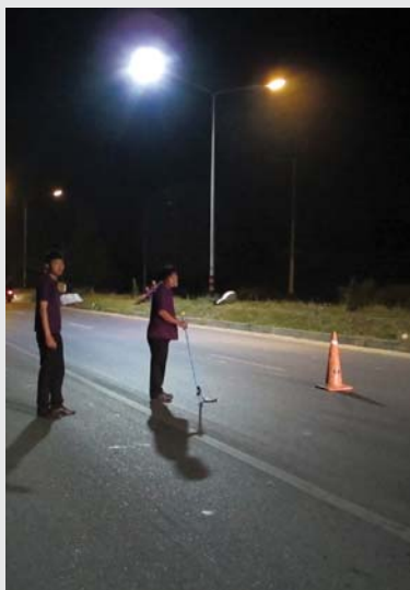
► Installation of Two LED Street Lighting Luminaires and Verification of Road Surface Illuminance
