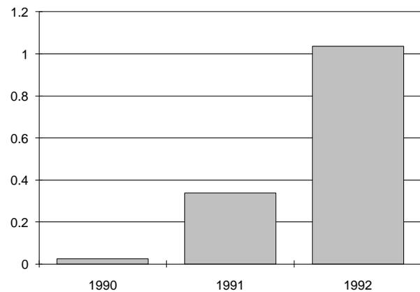
In 1992, the Irrigation Program resulted in energy savings of 411 MWh and lifecycle savings of 6,165 MWh. Capacity savings in 1992 were 700 kW. The program had few savings during its early pilot years, and significant savings did not begin to accumulate until 1991. Between 1990 and 1992, annual energy savings totaled 594 MWh, and capacity savings were 1.037 MW.
