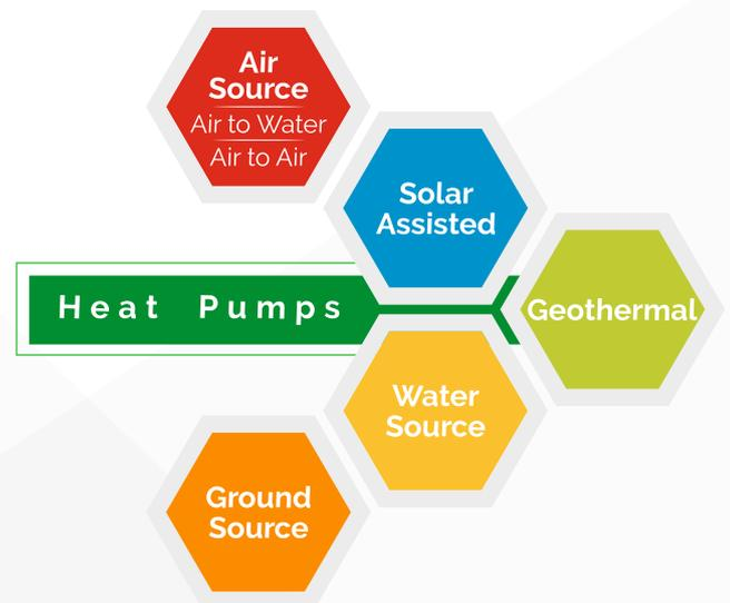
An air source heat pump (ASHP) takes low grade heat from the air, and boosts it to high grade that can be used for domestic heating or any other purpose. The pump uses less electricity than the heat it produces. The performance of an ASHP is similar to a refrigerator, but works in a reverse mode. ASHPs find applications in domestic space heating and hot water supply.
